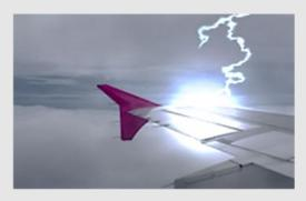
Each US aircraft is hit with lightning more than once a year. Aluminum allows the energy to travel along the skin and release back to the atmosphere. Composite structures cannot do this nearly as well and the potential exists for arcing close to fuel lines.
